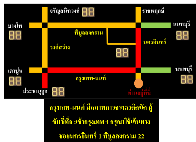
Figure 3.3-6 An Example of an Intelligent Traffic Sign Together with VMS for Introducing the Alternate Route
