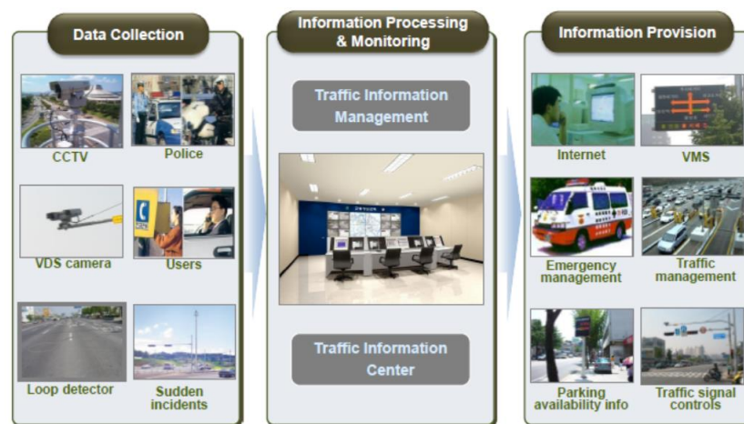
Figure 2.3-14 Advance Traffic Management System (ATMS)
