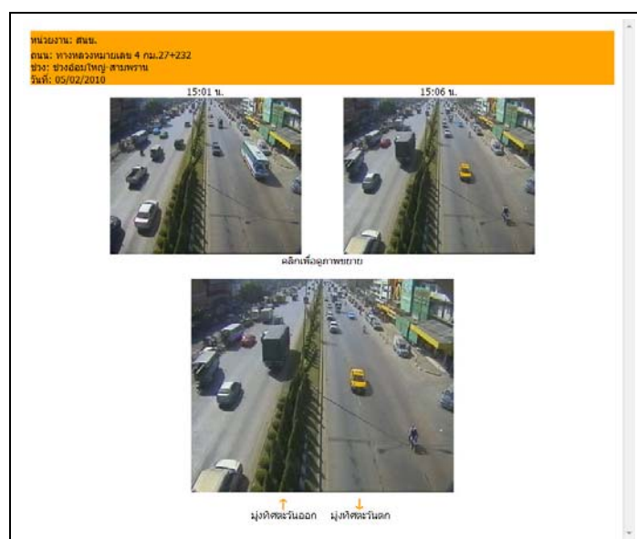
Figure 14 Sample of Information Dissemination System Connected from CCTV Installed on Highways in a Format of Still Picture
