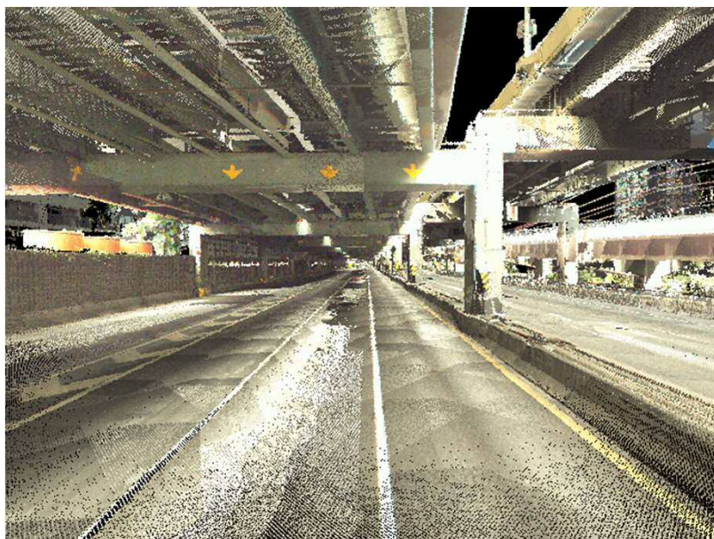
Example of 3D Point Cloud Data (EXAT)
